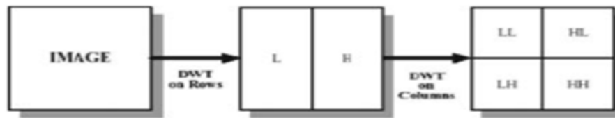
Figure. 2 : This image represents how DWT algorithm gets applied on Rows and Columns of an Image
