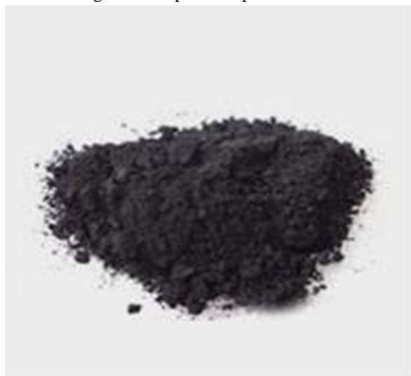
Fig 4. Water chestnut shell after activation
