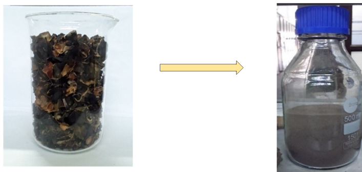
Fig 2. Water chestnut shells before and after crushing and grinding
