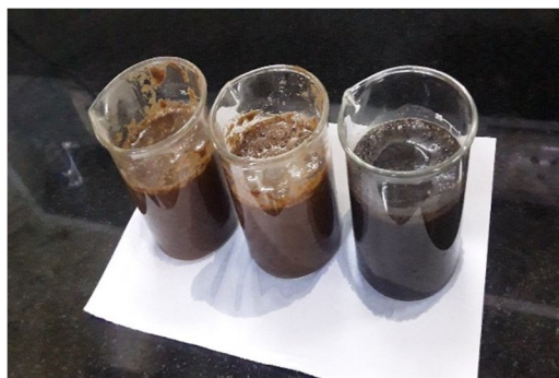
Fig 3. Water chestnut after impregnating with H_3PO_4
