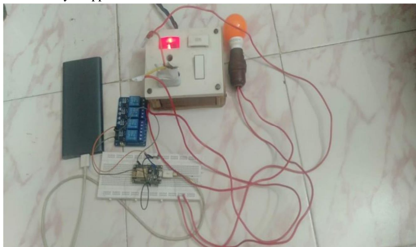
Figure: Output when the corresponding RELAY is turned OFF on blynk application
