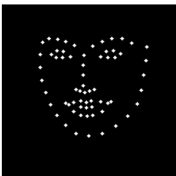
Fig 4. Facial landmarks for Eye detection.
