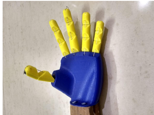
Fig.3. 3D printed palm of the prosthetic arm
