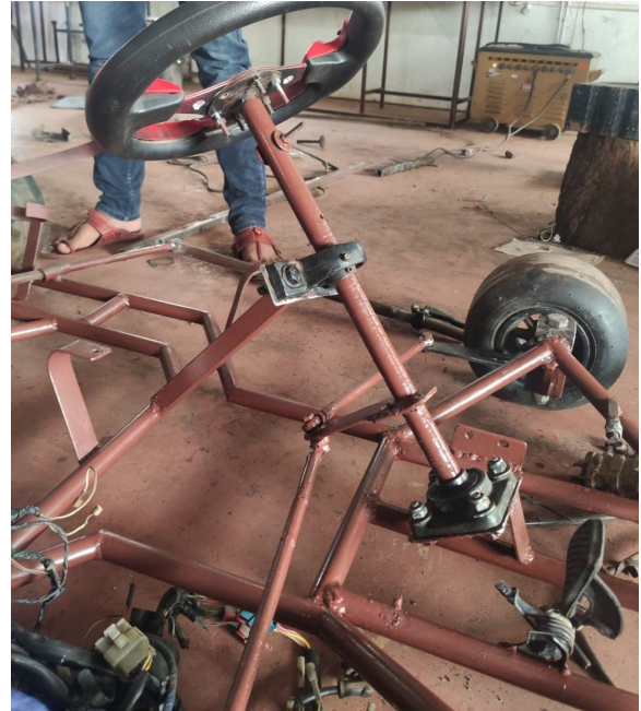
Fig..1 steering system using tie rod linkages
