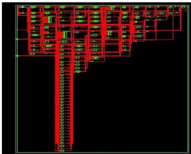
Figure 3: RTL Schematic of PMBIST
