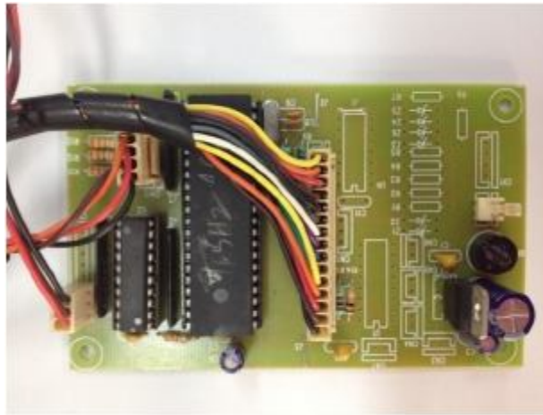
Fig. 7. PCB showing buffer, microcontroller and power supply
