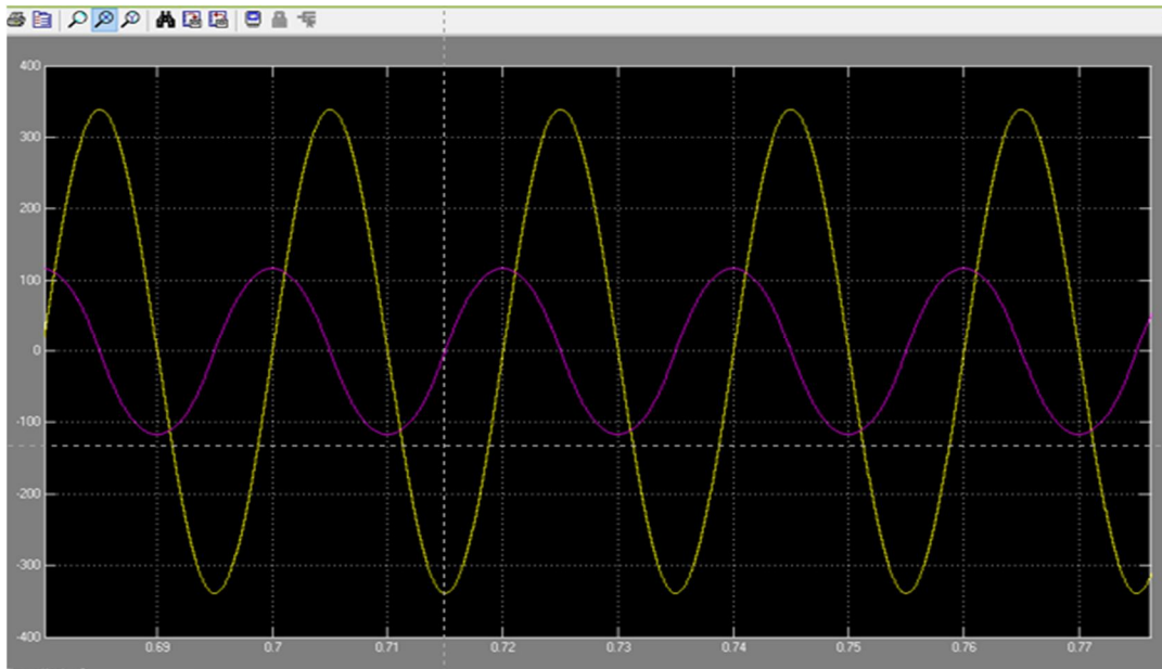
Fig.9 Voltage & Current waveform without STATCOM
