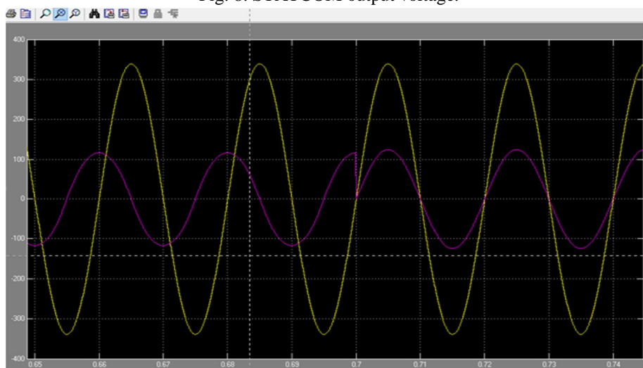
Fig. 9. Supply Voltage and Current at PCC.
