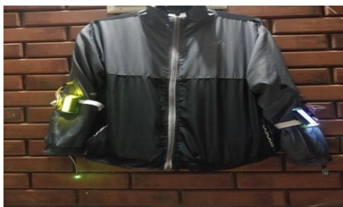
Fig : jacket with all the sensors attached.
