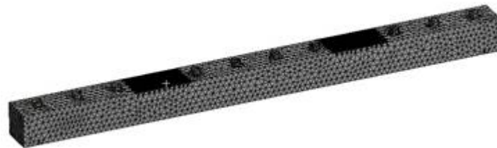
Fig 2 Mesh model of sandwich beam
