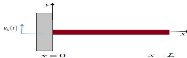
Figure 2.1: Cantilever beam excited by the motion of its base in the transverse direction
