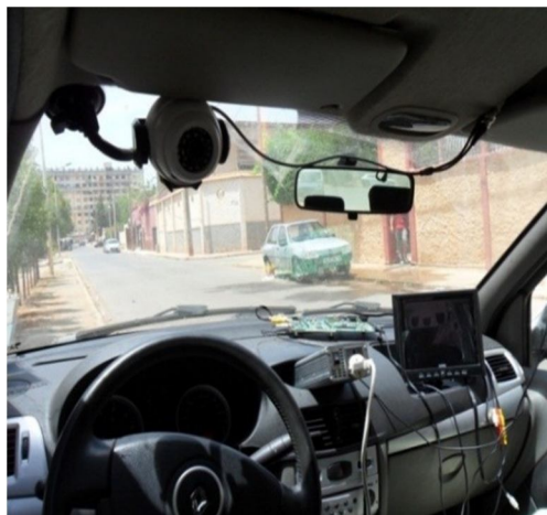
Figure 6 - Our system installed in the car based on IR camera
