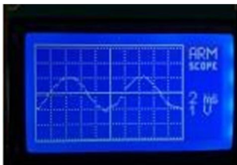
Figure 6.1: 2V and 100Hz Sinosodal Wave
