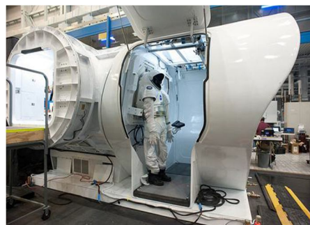
Fig 7: Suitports on the outside of the Multi-Mission Space Exploration Vehicle (MMEEV)
