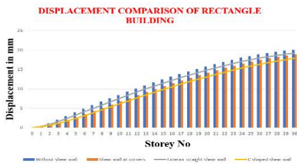
Fig:12 Storey Displacement of rectangle building.
