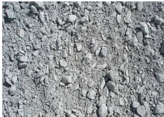
Figure 3. Recycled Aggregate as Granular Sub Base
