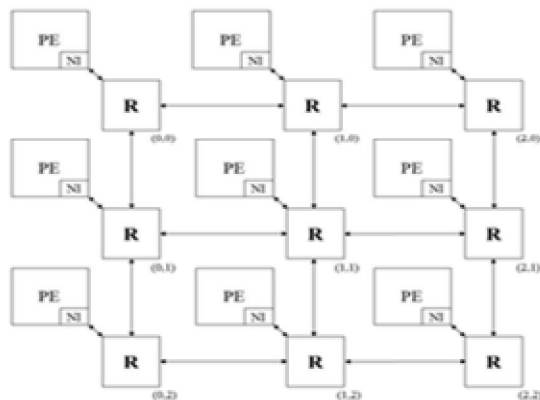
Fig.1. General Architecture of 3X3 NoC communication
