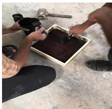
Fig.6 Greasing the mould
