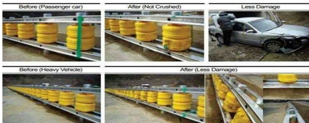
Figure.4.2.2. Crash test for car and truck collision at RB (KSI Korea)
