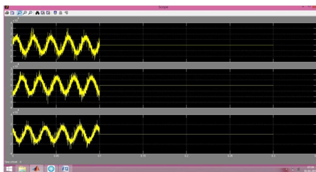
Figure 4: Waveform of three-phase fault voltage.
