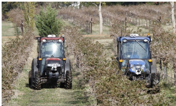
Fig. 7 Two autonomous tractors performing a spraying function. ASIrobots
