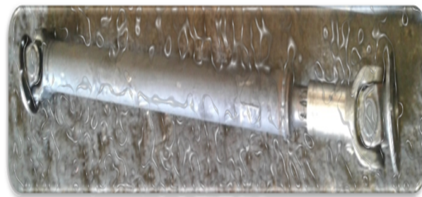
Fig-1.1: Universal Yoke Joint and Transmission Drive Shaft (Midi-712)
