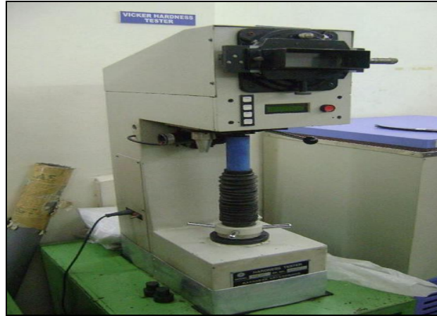
Figure 5.8 Vickers hardness test in urja laboratories.
