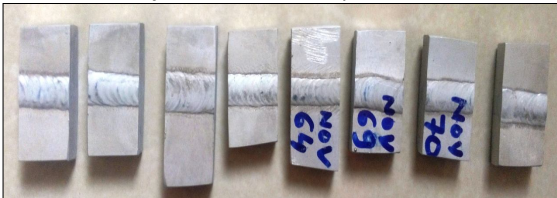
Figure 5.9 Vickers hardness Test Specimen As Per (IS:1500-2005)
