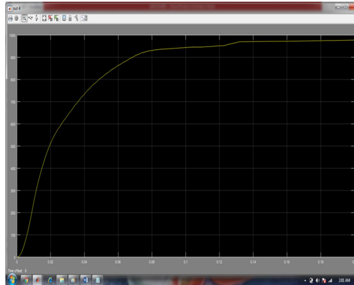
Fig (6.2) Transient response of Microgrid.
