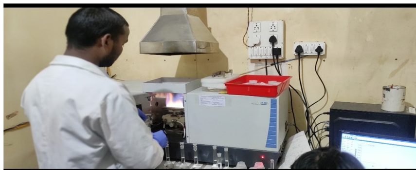
Fig: Atomic Absorption Spectrometer(AAS), running the water sample
