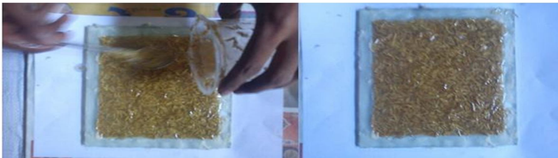
Figure 3.4 . Pouring the Bamboo Epoxy mixture on the glass mould.
