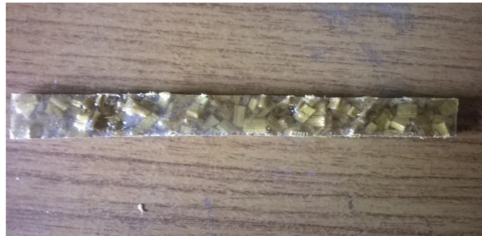
Fig 4.5 Specimen before Flexural Test
