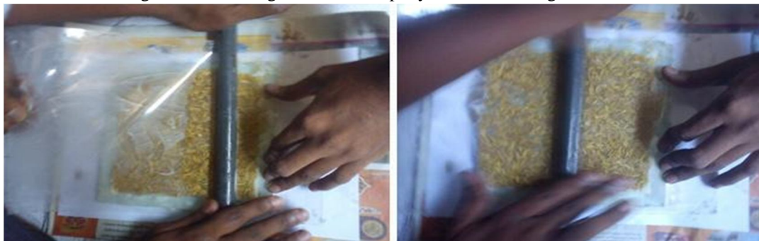
Figure 3.5 . Rolling on the surface of the specimen with a roller by keeping OHP sheet.
