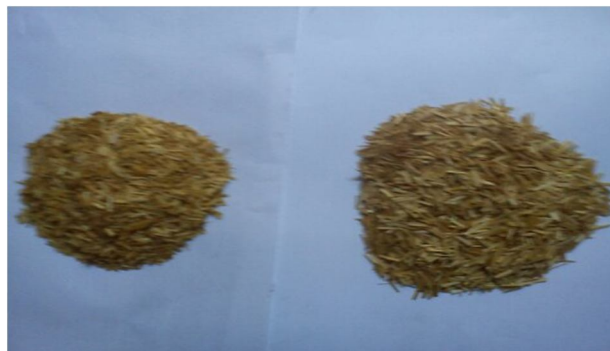
Figure 3.2 Chopped Bamboo fibers in 5 and 7mm lengths.
