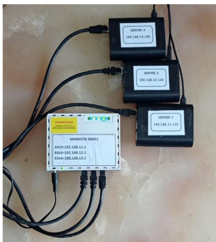
Fig. 2 VoIP Server with Raspberry Pi 3
