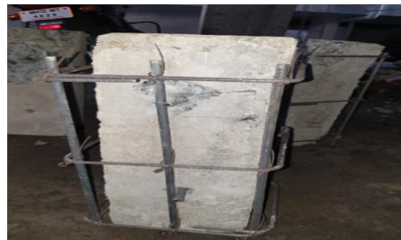
Figure 5: Virgin specimen with concrete jacket
