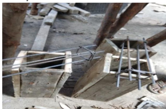
Figure 2: Mould & Reinforcement for virgin Specimen
