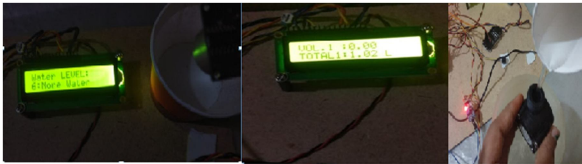
Water level sensor
