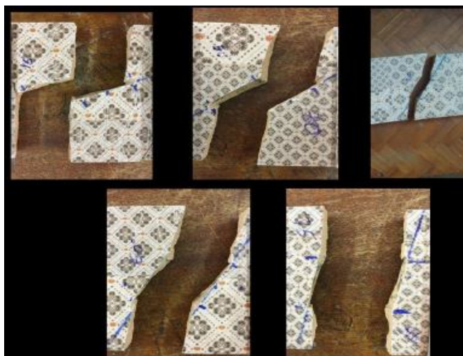
Fig. 3 Cracked brittle specimens with various inclination angle
