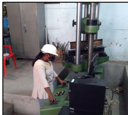
Fig. 8 Beam testing in UTM
