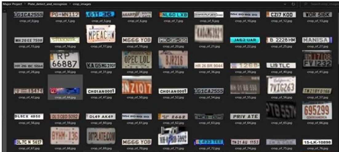
Fig. 3 Licence plates obtained from yolo model output
