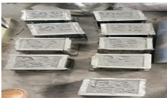
Fig no: 4.3 After removing the voids cube moulds
