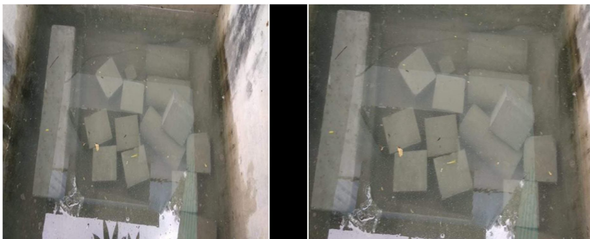
Fig no: 4.6 water curing
