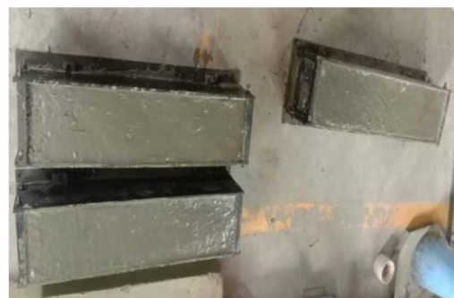
Fig no: 4.4 Placing of moulds in surface
