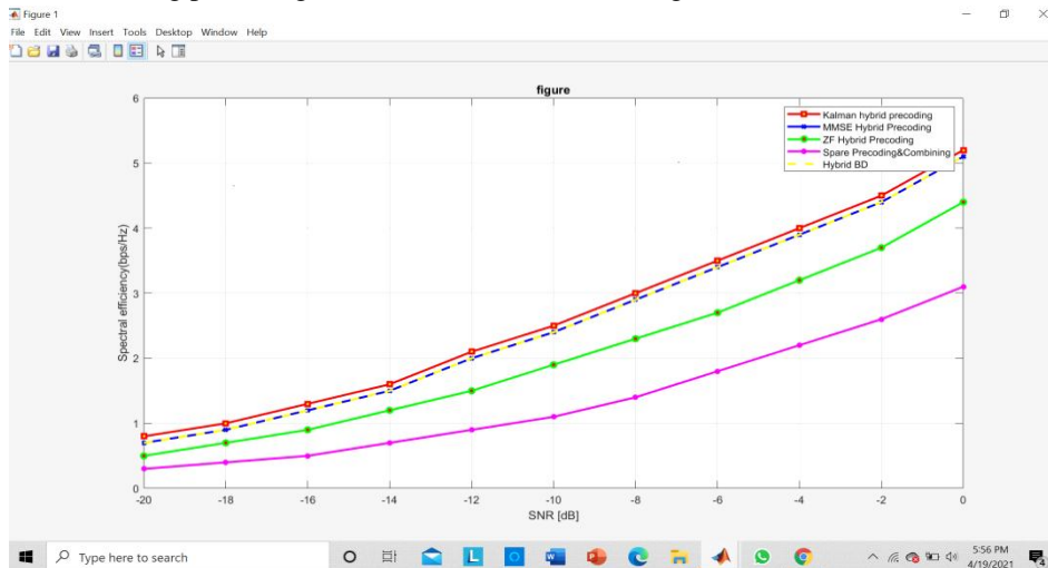
Fig. 4 Simulation results of Spectral efficiency vs SNR
