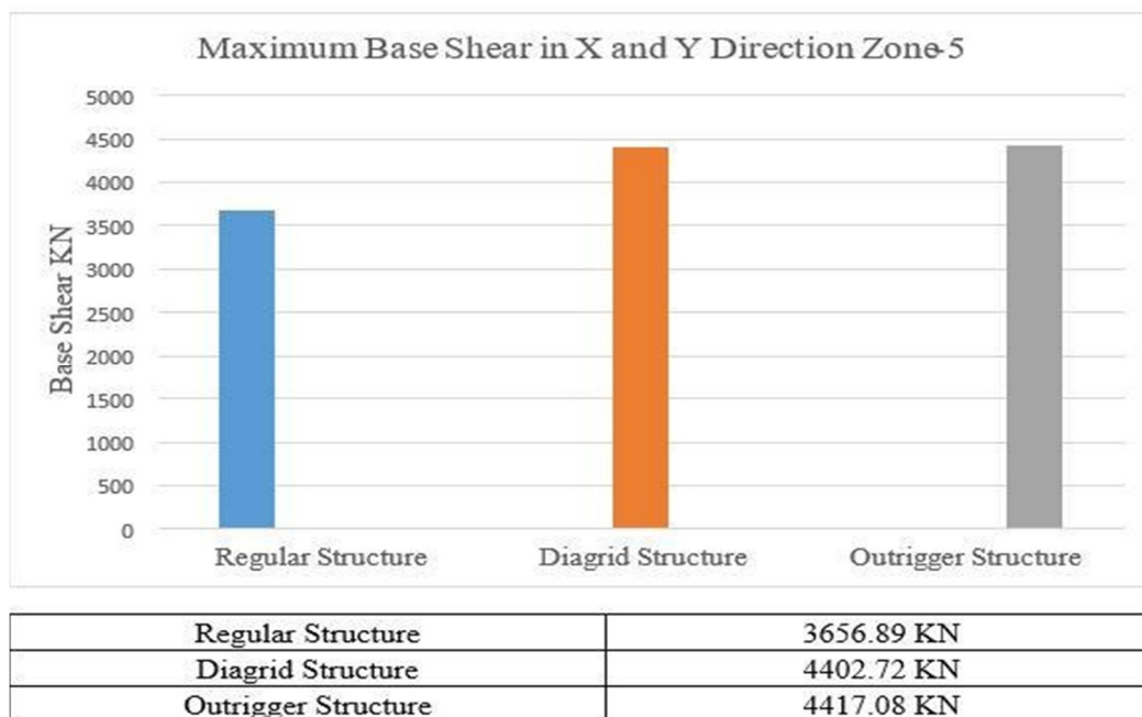
Fig 12. Maximum Base Shear X and Y Direction Zone 5
