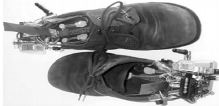
Figure 6. Shoe-integrated wireless sensor system, GaitShoe [5], showing all the hardware components.
