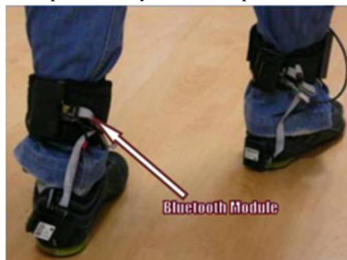
Figure 7. A wireless systems for gait and posture analysis based on pressure insoles and inertial measurement units [6]
