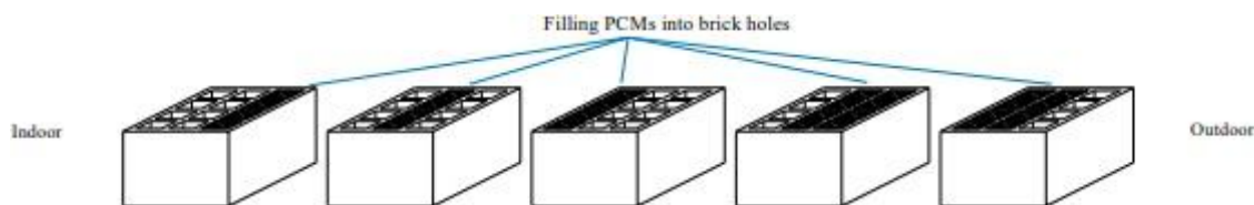
Fig 1. : Bricks filled with PCMs
