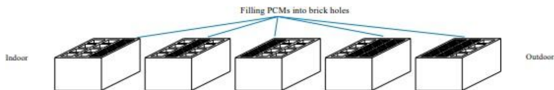
Fig 1. : Bricks filled with PCMs
