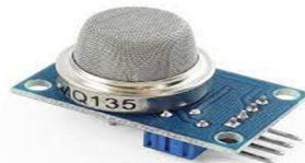
Figure 7: Air quality sensor (MQ135) for detecting a wide range of gases, including NH 3 , NO x , alcohol, benzene, smoke and CO 2
