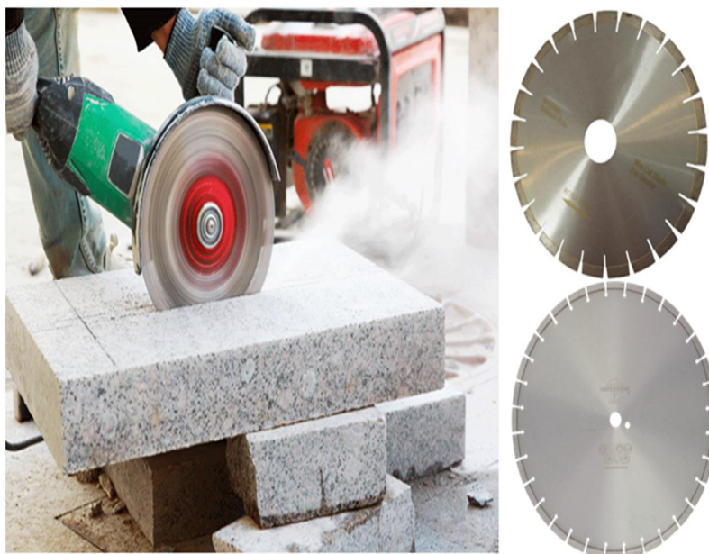
Fig 7: Figure shows the cutting operation of marble stone with two different diamond tool blades with same segments.
