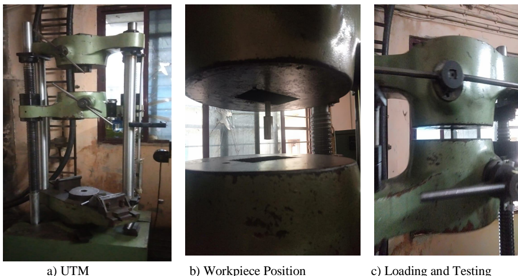
Fig. 9 Tensile Testing of Welded Joint on UTM 400 kN
