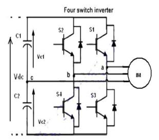
The PWM signal is applied to the switches to obtain the desired switching pattern and hence the desired output. To make this possible we employ the space vector pulse width modulation.
