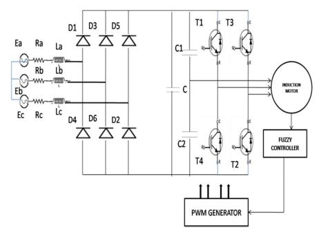
Vector control strategy is widely used in the implementation of four switch three phase inverter.
