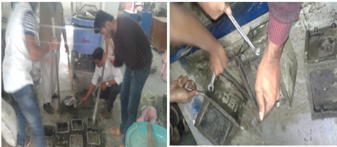
Fig. Preparation of Pervious Concrete Cubes
