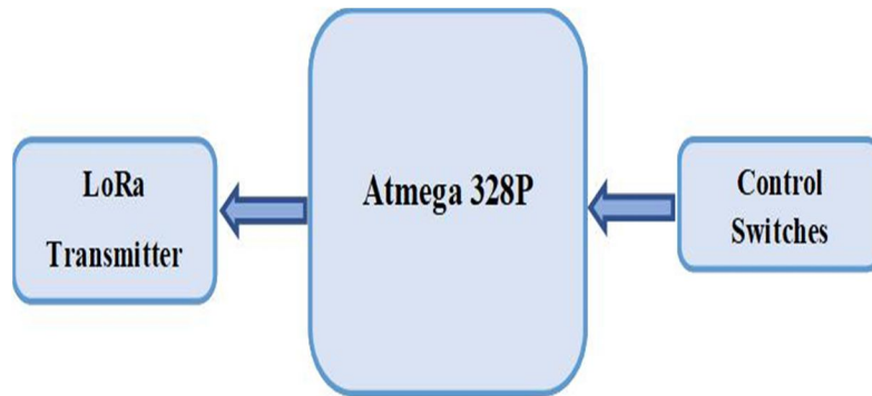
Fig. 1 Transmitter section block diagram
