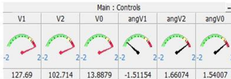
Figure 6 Measurements obtained for A-G fault
