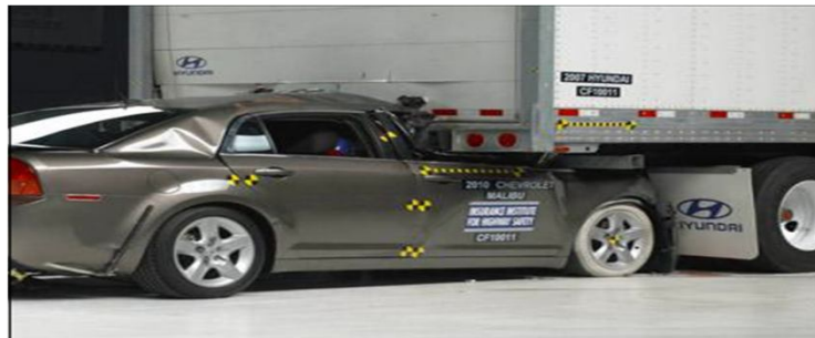
Fig. 1: Underride Crash of Car
