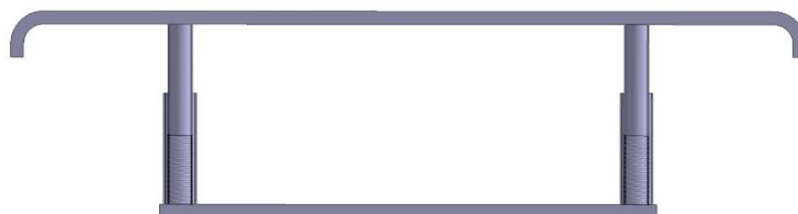
Fig12: Section View of Catia model of Safety Guard
