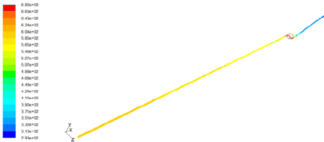
Fig.5 Temperature contour of Cu base wall
