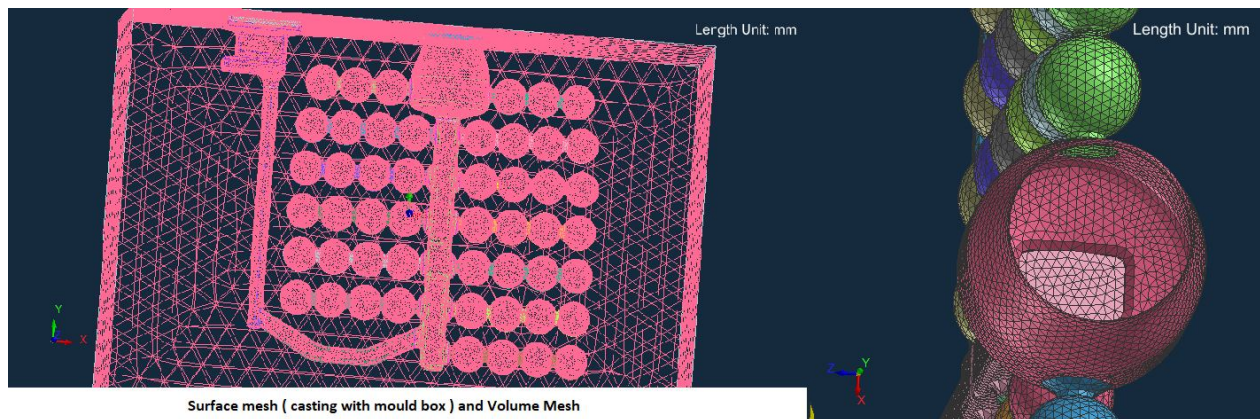
Fig. 5 Generated surface and volume mesh
