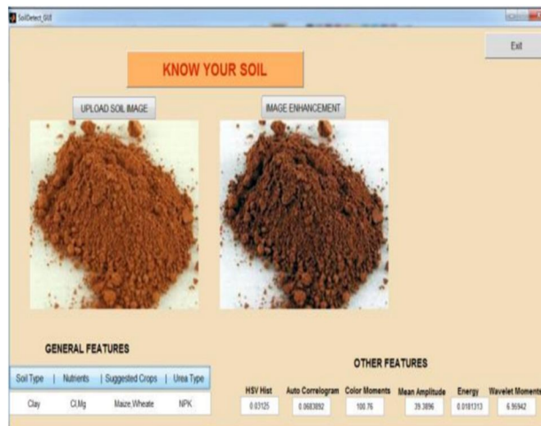
Fig. 4. HSV & Linear SVM based Soil Classification [9]
