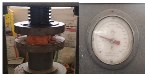
Fig 8: Compressive strength test conducted on brick
