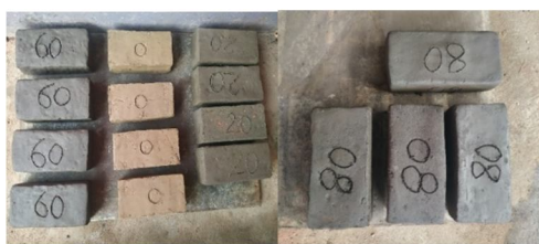
Fig1: Bricks kept for drying
