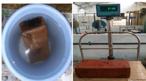
Fig 9: water absorption test conducted on bricks
